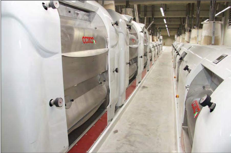
Above: The mill is equipped with 27 OCRIM rollstands (five double-high and 22 single-high). Right: The fifth or sifter floor includes six Great Western plansifters, five eight-section and one six-section for rebolt, with aluminum lift-out trays.
