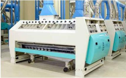
Among the equipment installed at Doruk Marmara Un Sanayi's new mill in Tekirdag, Turkey by Ugur Makina is this purifier. Photo courtesy of Ugur Makina.
