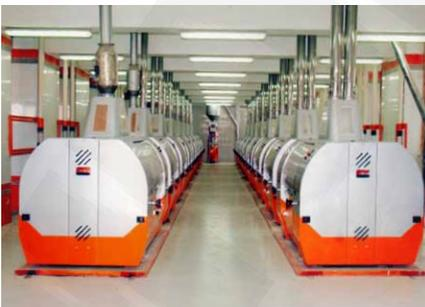
IMAS installed 16 roller mills at Union Friends Flour Mills' new plant in Asyout, Egypt. Photo courtesy of IMAS.
