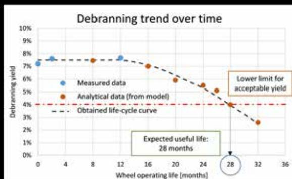
Figure 7 - Graph of the debranning trend over time for a diamond wheels debranning machine.
