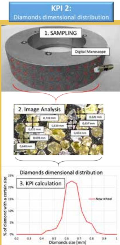
Figure 3 - Diagram of the procedure used to calculate the KPI2. Another important aspect that influence the debranning
