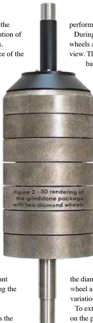
Figure 2 - 3D rendering of the grindstone package with two diamond wheels
