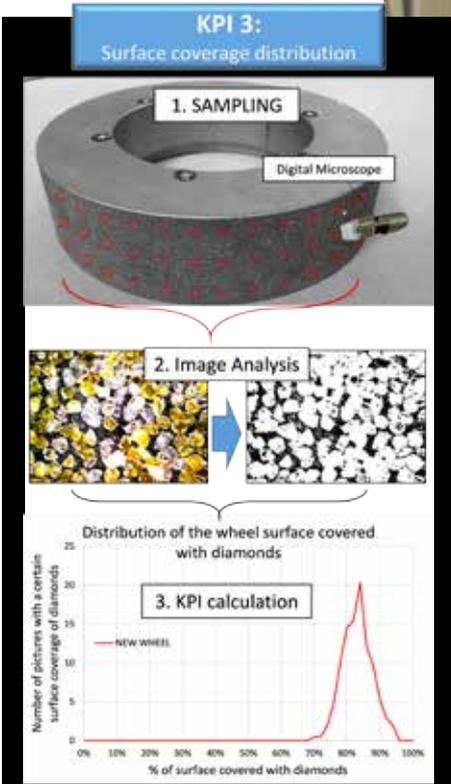
Figure 4 - Diagram of the procedure used to calculate the KPI3. The indicators were very important to quantify the wear process of the diamond wheels over time
