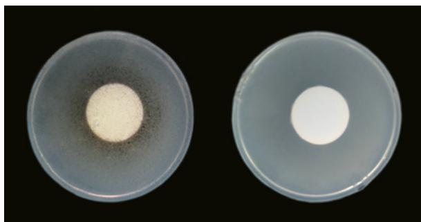
Microbiological test on a wood frame (left) and the new antimicrobial frame material (right) (Ocrim).
